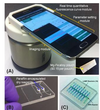
**Fig. 4. Prototype of a highly multiplexed, miniature, field-deployable, sample-to-answer molecular detection system capable of co-detecting soil-borne pathogens.**
